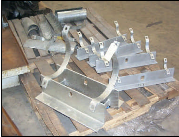
Small Diameter Clamped Shoes fabricated to be assembled into Pre-insulated Supports
