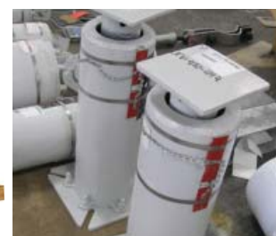
CHAINED TRAVEL STOPS ON VARIABLE SPRING SUPPORTS
